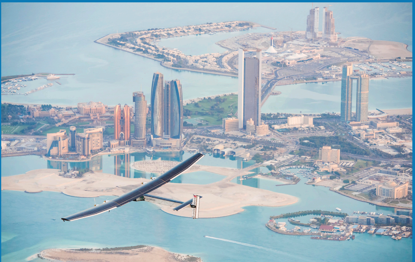
Figure 6. The Solar Impulse 2 has a carbon-fibre body covered with 17,248 solar cells. Source: Masdar
