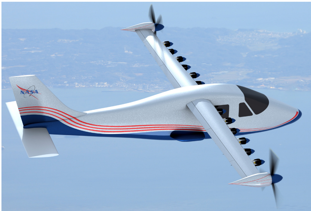
Figure 1. X57 Maxwell all-electric aircraft under development by NASA. Source: Allard, 2016
